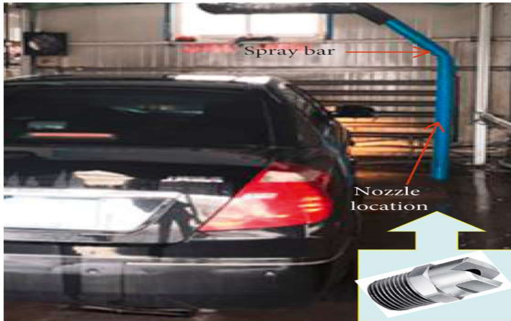
Fig 3 : The physical diagram of the side spray bar of an automatic automobile washer.
